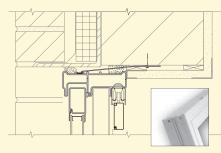
**BLOCK FRAME** (WITH CLIP ATTACHMENT) Masonry openings or pocket replacement.
